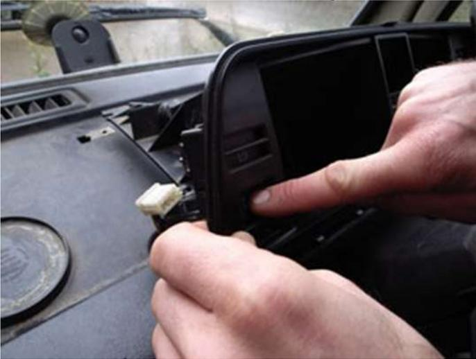
**7. Remove the rest of the switches from the cluster.**
