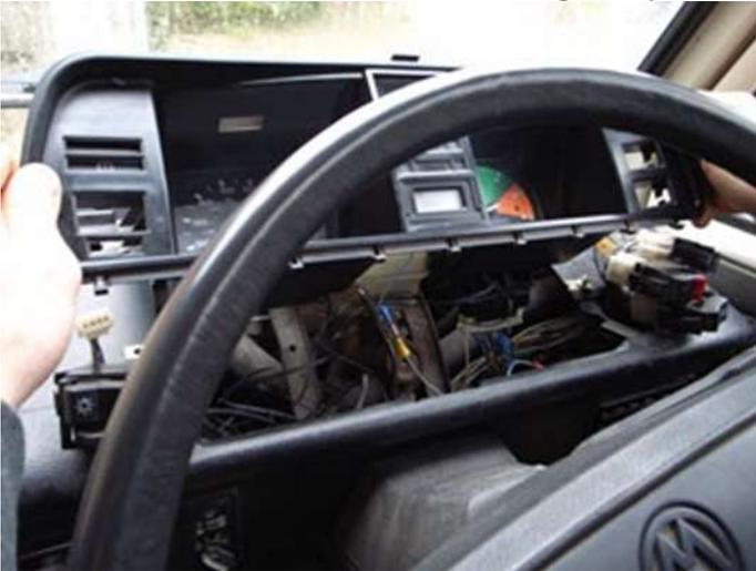
10. Unplug the multi pin connector from behind the tachometer.
