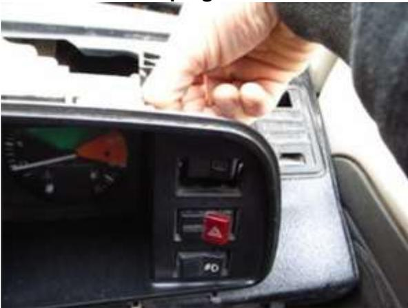
**5. Loosen, but do not remove the last screw - this will enable you to remove the cluster by sliding it sideways with the screw still in place (the screw is very easy to lose otherwise).**
